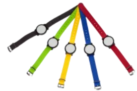
Passive (125 KHz/13.56 MHz) and active (2,45 GHz) RFID tags
